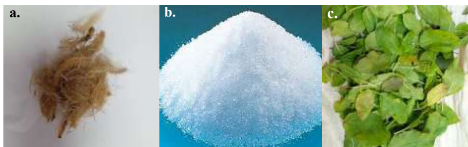
Figure 1: Primary raw materials used for bioplastic film preparation: (a) AHF, (b) PVA resin, and (c) Tulsi leaves.
