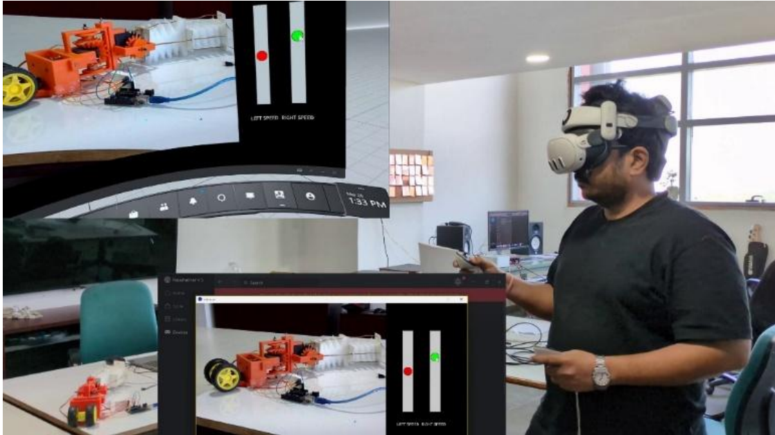
Figure 3: The mixed reality experiment in progress. The top left insert shows the point of view of the user through the VR headset. The snake robot that was being controlled is in the bottom left.
