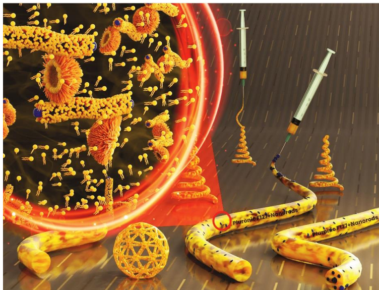
Figure 1: Composite hydrogels containing small amounts of paramagnetic akaganeite ( \beta -FeOOH) nanorods in PF127 triblock copolymer show enhanced thermal stability and injectability which could find applications in tissue engineering and drug delivery.
