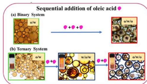
Figure 1: Emulsions stabilized by sequential addition of oleic acid in binary system (a) and ternary systems (b).
