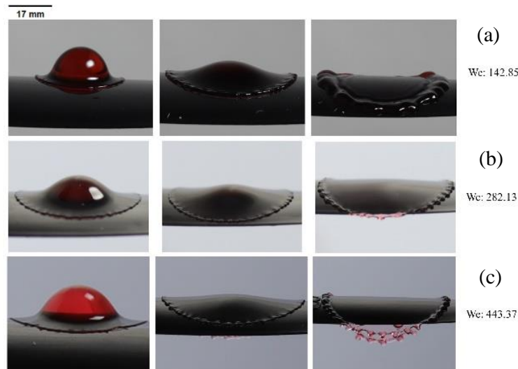
Figure 1: Droplet impact on the static propeller at the mid-section of the propeller for droplets dispensed from three different heights (a) 20 cm, (b) 39.5 cm, and (c) 62 cm.
